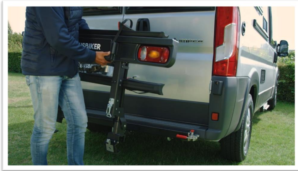
Step 1: Loosen the screws at the back.
