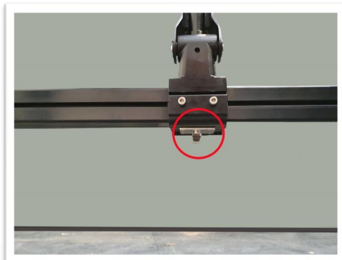
Step 2: Loosen the screw at the bottom.
