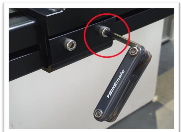
Step 1: Loosen the screws at the back.
